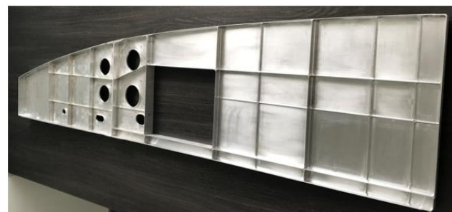
Fig. 5. Chassis beam made using the HSM method with two integral parts. HSM, high-speed machining
