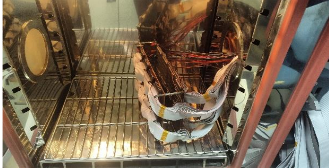
Fig. 8. PCBs in a thermal chamber. PCB, printed circuit board
